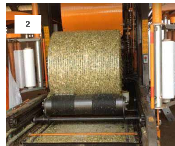
Wrapping the crop with net in the pre-final phase of silage manufacturing
